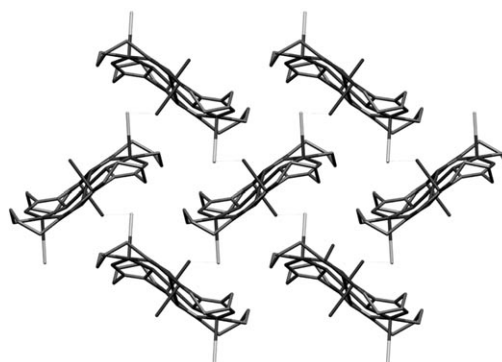
Figure 5. Stick representation of the metallacrown units in the crystal, projected down the crystallographic a axis. The neutral complexes are arranged in a herringbone mode and interact with each other by means of O1w \cdots Cl1 hydrogen bonds.
